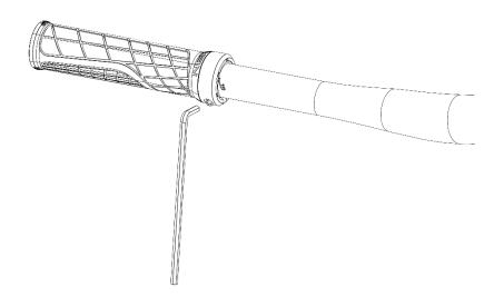
Once the desired width has been set, the handle must be tightened to a torque of 3 Nm.
