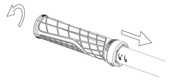
Never attach the handlebars outside the "STOP" mark. This must be covered by the grip.
